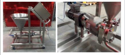
Trolley mounted Unibloc Rotary Lobe pump with tungsten carbide mechanical seals on a mobile frame, fitted with a pillow plate jacketed hopper. It has a control panel with variable speed drive and touch screen controls.
